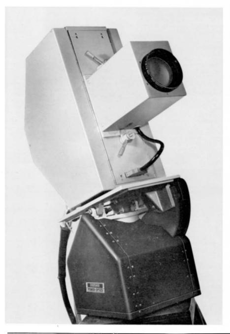
Fully remote-controlled camera system with servo-operated lens drive
