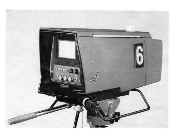
Equipment Type **CO 301** is a camera unit intended more particularly for use in the open. Its light weight, small dimensions, low consumption, insensitivity to microphonic effects are especially valuable when used on a coach, a light OB van or a helicopter.
