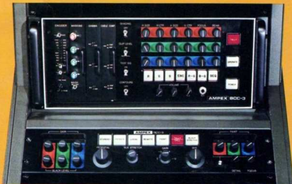
The BCC-3 camera control unit, with close up view of the controls.
