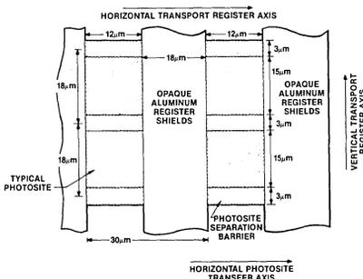
NOTE: Photosite Separation Barriers are transparent, photosites are optically contiguous along the vertical axis.
