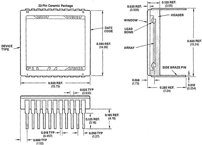
NOTES: All dimensions in inches (**bold**) and millimeters (parentheses). Header is black ceramic ( $Al_2O_3$ ). Glass window is attached to header with epoxy cement.
