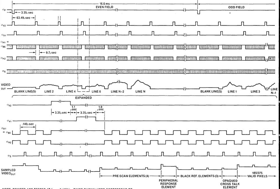
NOTE: DEVICES ARE TESTED AT  $f_{clk} = 7.16\text{MHz}$ . TIMES SHOWN HERE CORRESPOND TO THIS CLOCKING FREQUENCY WHICH IS NTSC COMPATIBLE.
