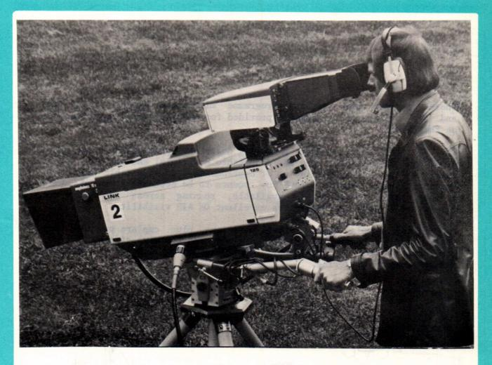
This new Studio/OB camera is based on the already successful 120 series Multi-mode camera and retains the comprehensive operational facilities for which Link cameras are well known.
