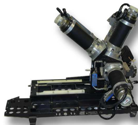
The camera chassis and scanning yokes.
