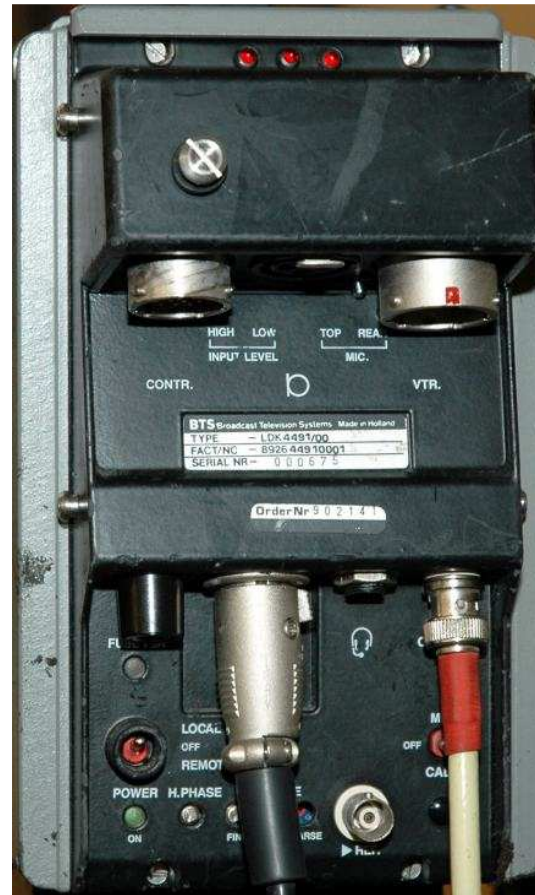
This is the rear of the EFP back with connectors for VTR and or CCU.
