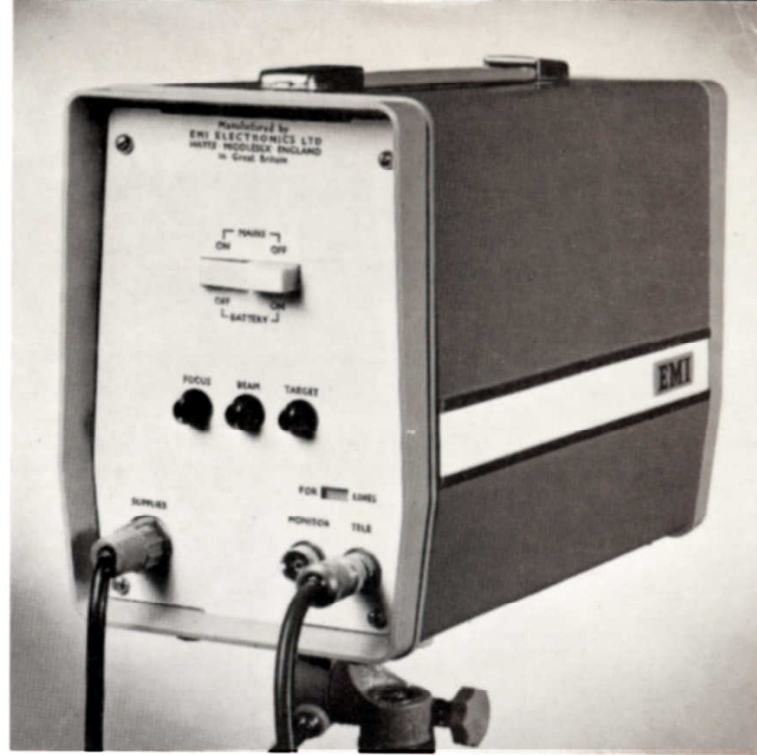
Rear view of camera showing controls and connections
