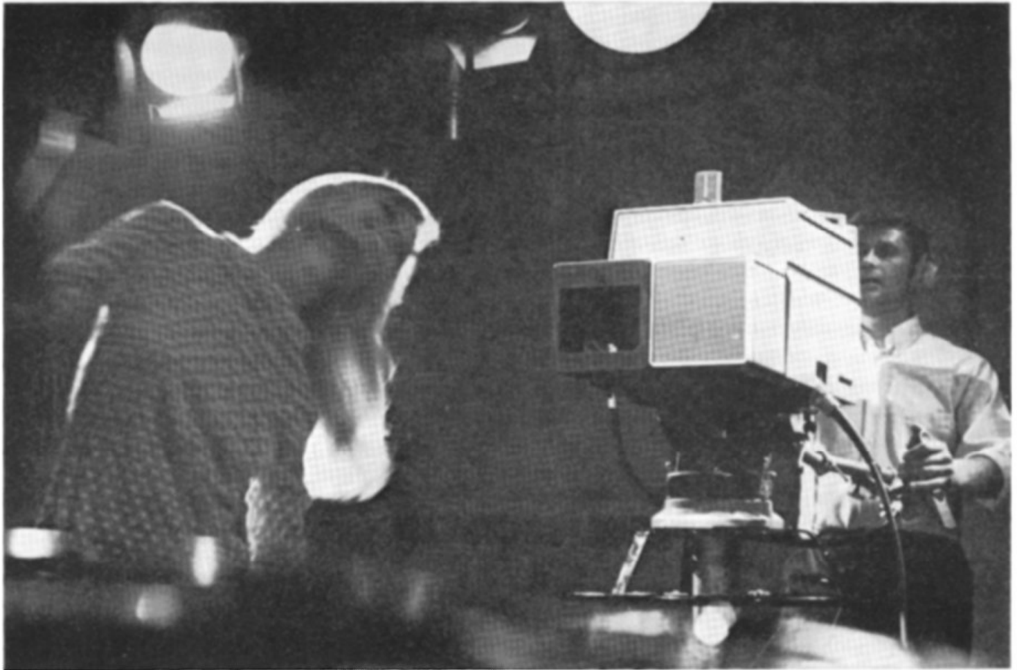
Handy Mark VIII – under 100lb working weight and 2 ft in length – uses \frac{1}{2} in. cable – compact CCU.
