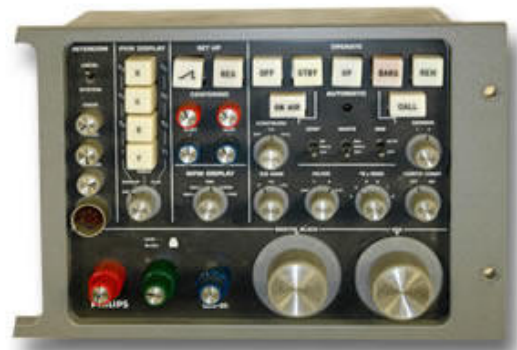
The control panel for the LDK15 & 25
