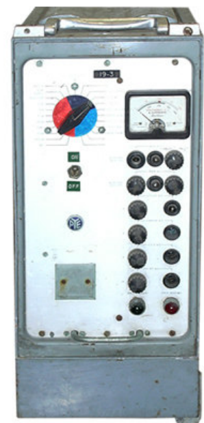
The Pye Mk6 PSU with switch, meter and fuses
