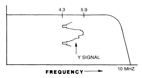
Note that no consideration need be given to such considerations as "highband" and "shelves," because the signal is pure monochrome; the strong subcarrier signals which have caused moire in past systems are completely absent.
