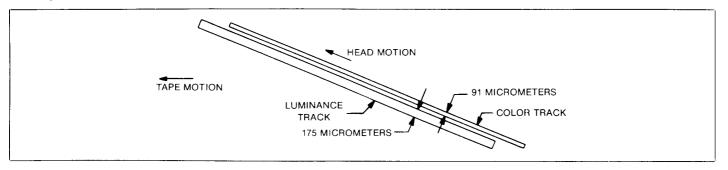
are written by a pair of heads very close to each other on the drum. Each of the two tracks is 9.4 cm long, and the two tracks, taken together, contain the information for a complete field of the video signal.
