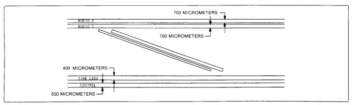
The primary audio tracks (Audio 1 and 2) are nominally 700 micrometers wide, with another 700 micrometers designated as the guard band between them. Audio 3, usually used for time and control code, has a 400-micrometer width, and is separated from the 500-micrometer control track by a 400-micrometer quard band.
