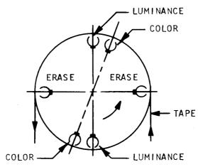
Note that, unlike Type C format, the drum rotation and tape motion are in the same direction. Although this costs about 3% in head-to-tape speed, the resulting smaller air film and better head-to-tape contact more than compensates for any response loss. Such conservative system design considerations make it possible to obtain a 4.0 Mhz luminance response at only 4.7 m/s head-to-tape speed.
