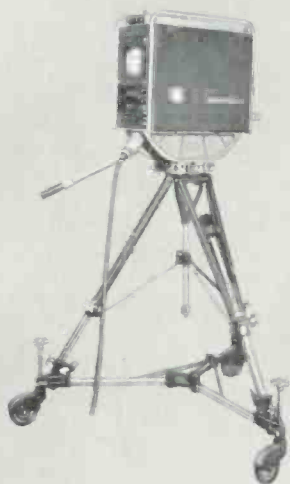
BASIC CAMERA CHAIN WITH LOCAL CAMERA CONTROLS
