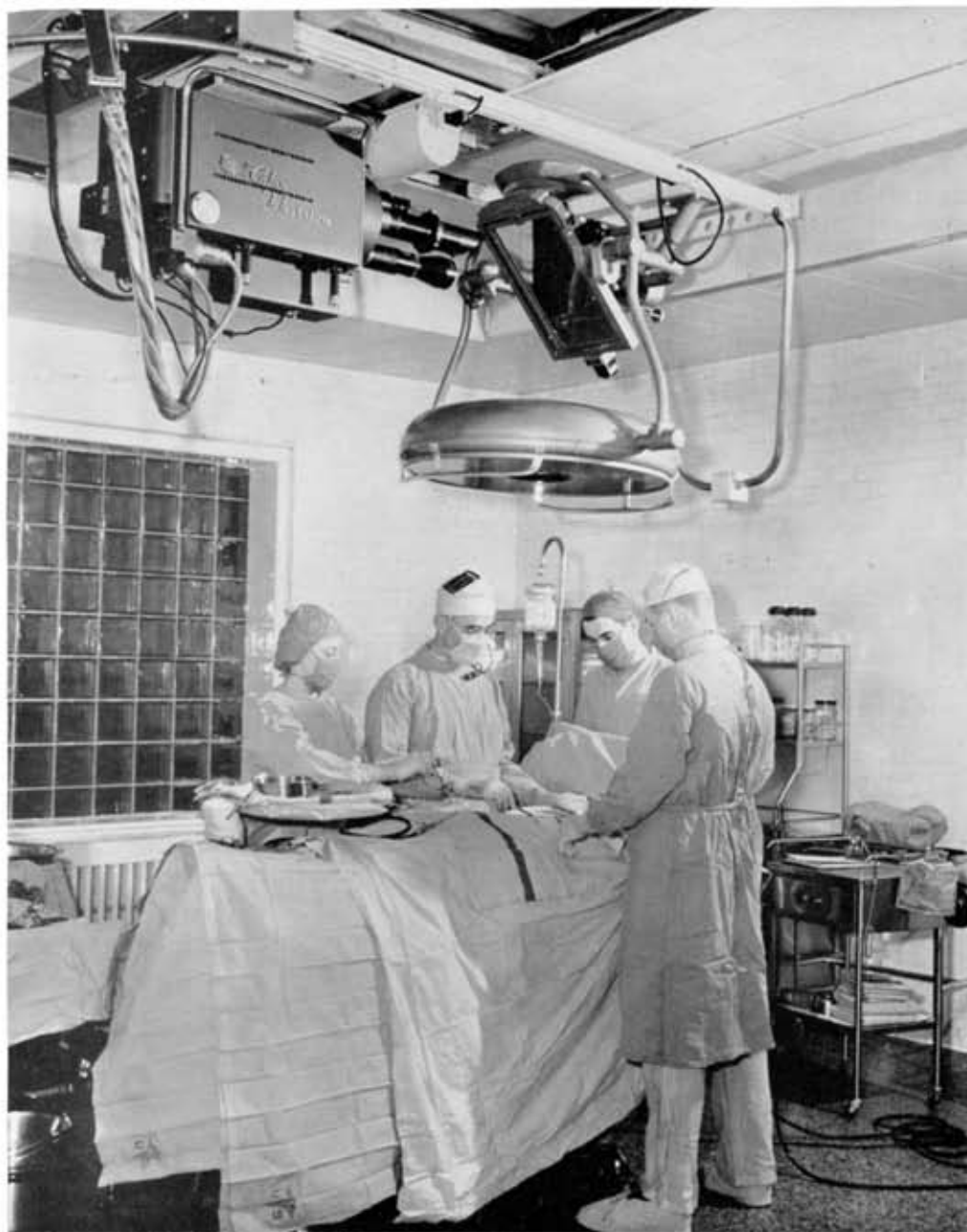
FIG. 15. TK-45 color camera suspended overhead and focused on the operating field by a special mirror.
