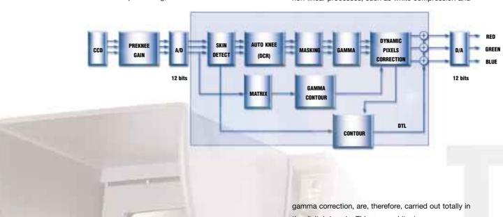
gamma correction, are, therefore, carried out totally in the digital domain. This new architecture ensures stability of camera adjustments together with excellent reproducibility between cameras.
